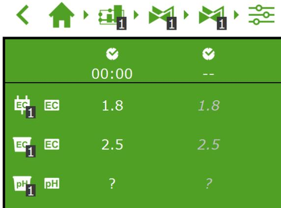
Figure 5-3: You can set the EC (and the pH) for each predefined period.
